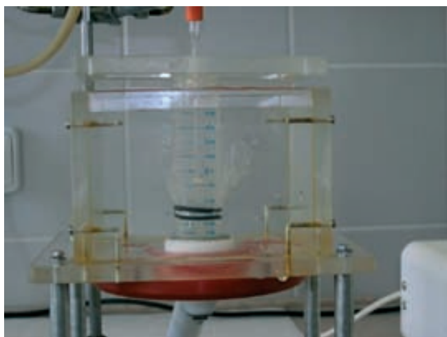
Fig. 3 Fixation of sonication head, plastic cylindrical vessel
