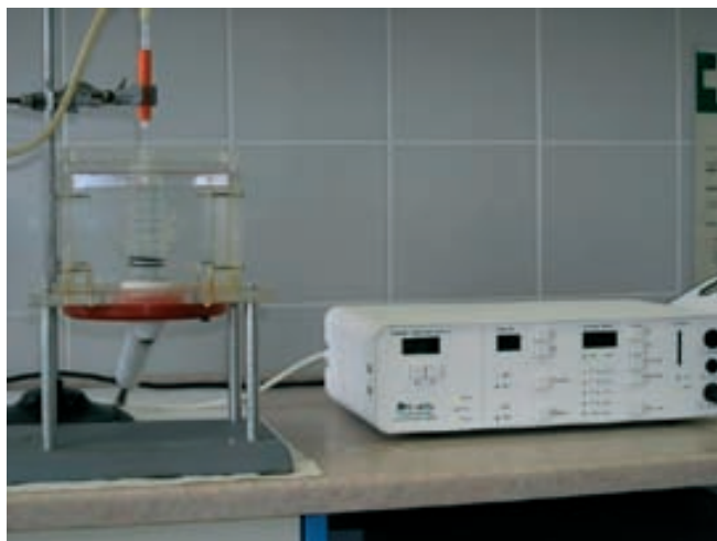
Fig. 2 Therapeutic ultrasound instrument BTL-07p
